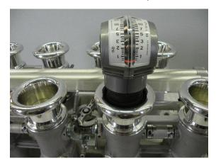
2.Next, disconnect the linkage rods at the center pulley by removing the 10-32 hex head screws
