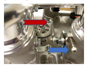
3. Back off throttle stop screws (Blue arrow). You cannot adjust the center compensating linkage unless you allow room for the throttle stop to move back.
